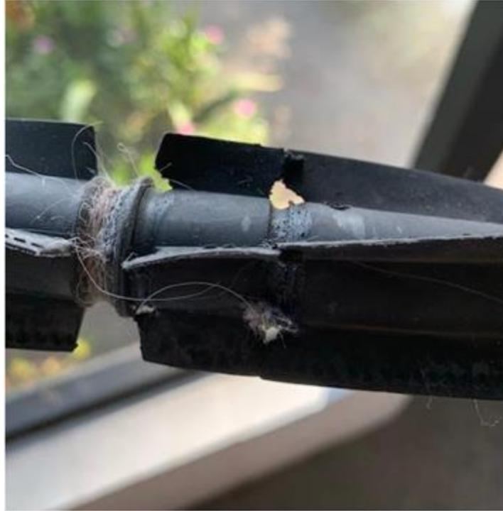
*Figure 3. “Self-cleaning brush roll with tangled hair and damage.*
