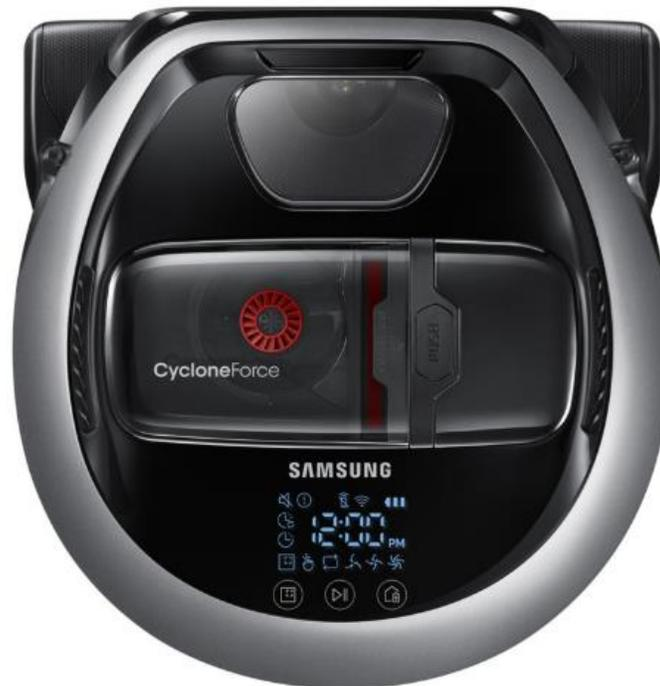
*Figure 2. Top mounted bin in Samsung R7065*
