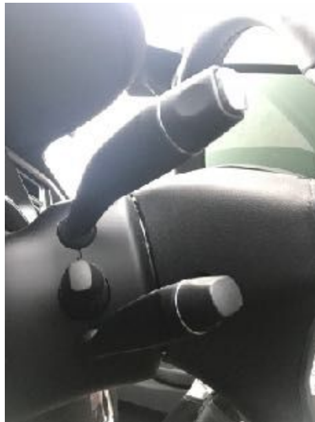
Figure 7. From top to bottom: windshield wiper stalk, steering wheel adjustment nub, and Autopilot stalk.
